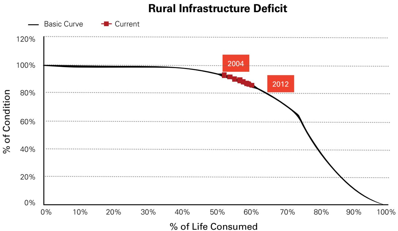
The preceding graph provides an example of the power of the deterioration curve. Here the condition of the culvert assets was modeled. The horizontal axis represents the average age of the infrastructure as a percentage of its lifespan (e.g., infrastructure at the end of its life would be rated 100%).
